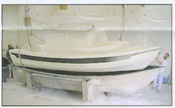
Hull and top deck are molded as separate parts and then fiber-glassed together while still in the mold to insure perfect alignment and to eliminate any possibility of twist. This construction method provides a very strong, rigid lightweight shell that is free of leaks or fatiguing joints. Color accent & top deck nonskid patterns are molded in.
