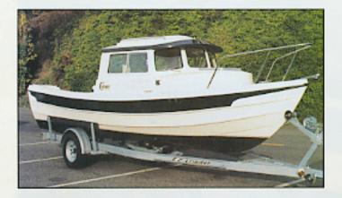
The 22' Angler (shown above) has the smaller house, giving more room to the aft deck (22"). The only feature change from the 22' Cruiser (shown below) is the omission of the galley and the dinette does not make into a berth.
