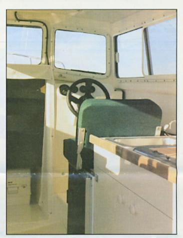
Interior trim is neat and utilitarian, lending to the boats easy maintenance. All cabinetry is removable and is made from marine grade plywood (3/4") with a protective plastic overlay. The exterior door and the foot-boards under the dinette and pilots station are of a solid plastic material called Starboard (similar to the plastic chopping board in your kitchen).
