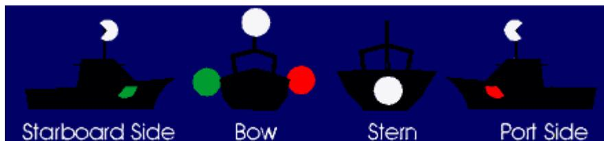
Does your stern light shine dead astern over the required 135° arc or does it shine to one side or up or down. Can it be seen from the required 2 miles and
