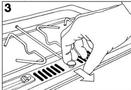
Make sure that flames are completely extinguished and that there is no heat-glow on top of the tanks, and then lift out fuel tanks.
