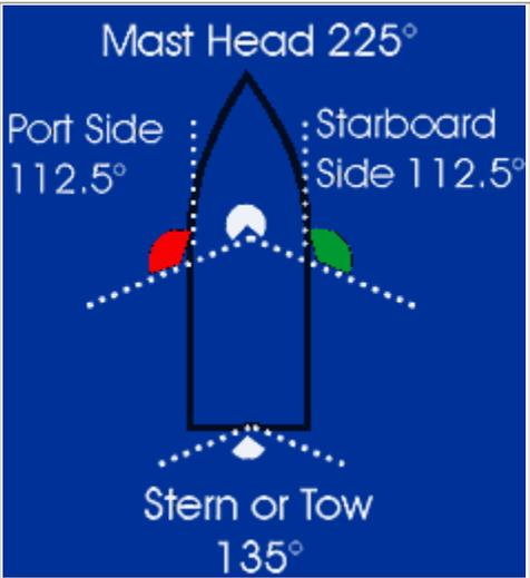
The arc of the lights and color allows you to determine the direction a vessel is moving. How good are your lights? You should test them to see how visible you might be at night. Whether on a trailer or at the marina switch on your lights and see how well they can be seen. Walk away from the boat or row away, if you are at anchor or at a mooring, and see how visible the lights are as you move further away. How easy are they to see against the background of lights on shore?
