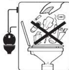
tampons or sanitary napkins. The holding tank and pump should be flushed with several gallons of water after each pumpout. Make sure the battery is fully charged. The dc motor is suitable only for intermittent duty and should not be run for more than 15 minutes continuously. At maximum flow
