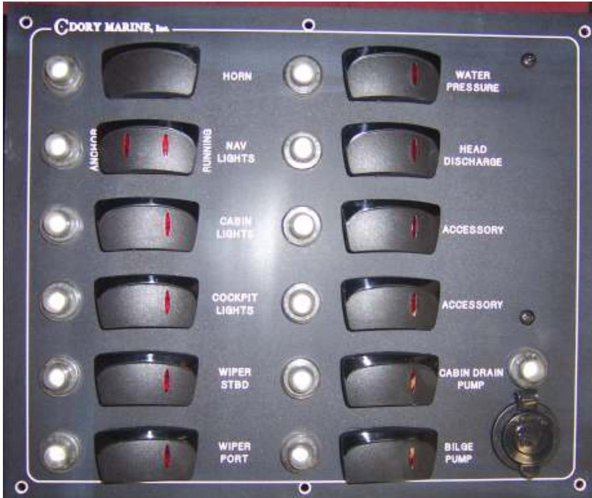
The Pilot Station Electrical Panel is located near and to the right of the helm. It contains circuit reset breakers, switches and 12 Volt Plug. The circuit reset breakers are white and round and are used to reset the circuit if needed. If a circuit breaker trips investigate the situation before pressing in the reset breaker.
