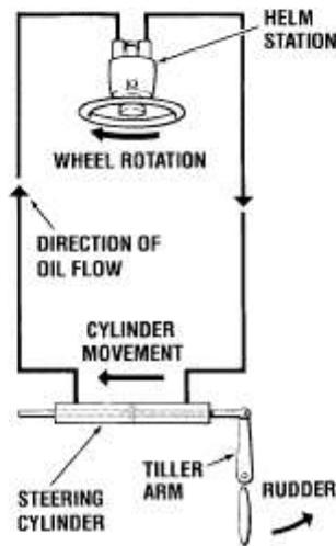
The system is a two-line system. This makes operation very simple.
