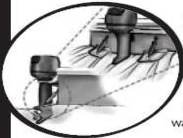
Bennett Trim Tabs are attached to the bottom edge of the transom. When the helm control is pressed, the trim tabs move into position. Water-force on the trim tab surface creates upward pressure, raising the stern and lowering the bow. Properly sized Trim Tabs improve the performance of your boat in a much wider range of weight, weather and water conditions.
