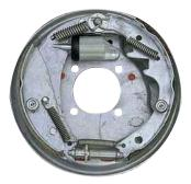
Fig 13: Hydraulic Drum Brakes
