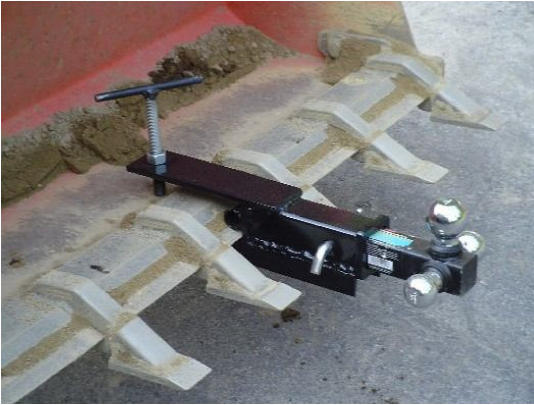
Finished receiver hitch mounted on bucket with toothbar.
