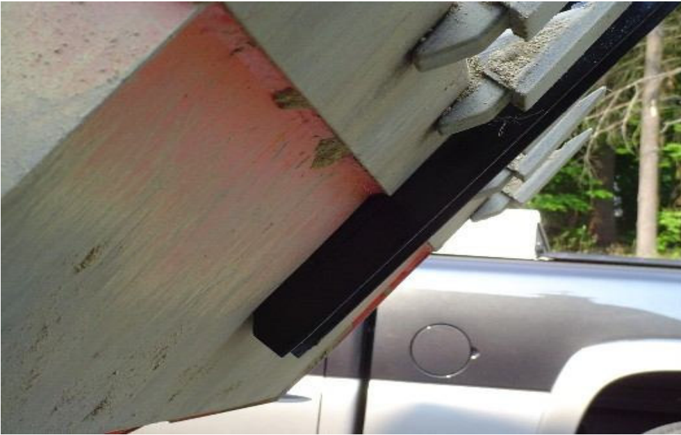
Close-up of bucket bottom showing the bottom pad up against the bucket cutting edge.
