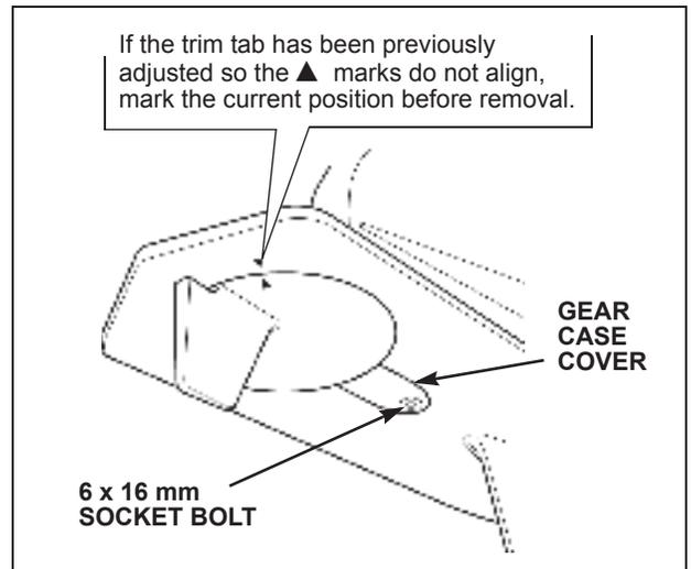
Remove the 10 x 80 mm bolt and washer, four 10 x 40 mm bolts and washers, and remove the gear case assembly. The vertical shaft will stay connected to the gear case, so remove the gear case without twisting, and then place the unit on a workbench.
