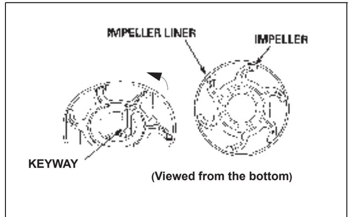
Insert a new greased O-ring and water tube seal rubber and four distance collars into the impeller housing. Install the pump liner/impeller into the housing.
