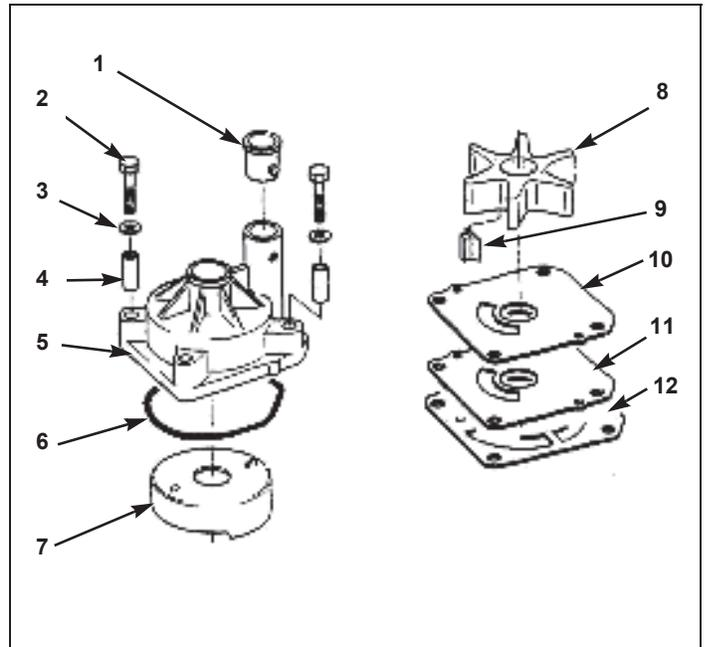
Start reassembling the pump by applying marine grease to the inner surface of the impeller liner, housing O-ring, and the water tube seal rubber.
