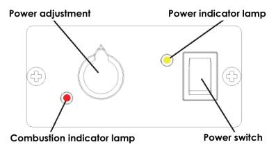
After starting, the power can be adjusted with the control rheostat. Avoid unnecessary rapid adjustments, as this can accelerate soot deposition.
