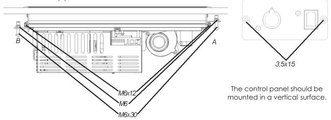
Figure 7: Attaching 85DP to mounting rails.
